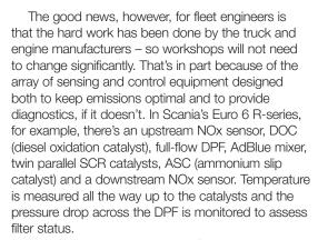
Here lies a potential niggle for fleet engineers, though. As mentioned above, the particulate filter will need to be cleaned at intervals corresponding to the truck's duty cycle. As has been found in some PSV (passenger service vehicle) applications, a stop-start regime - or any departure from long-haul work stresses the system. So care may be needed to avoid a build-up of ash that could overtake the capacity of the regeneration process.
